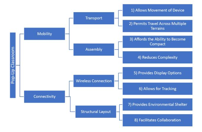
The two systems that define the purpose of this device are mobility and connectivity. Mobility defines the nomadic aspects of the project as well as the associated moving parts. This includes transportation components and assembly aspects. Connectivity defines the experiences connected with promoting collaboration and providing typical components of the educational experience. Underneath this
