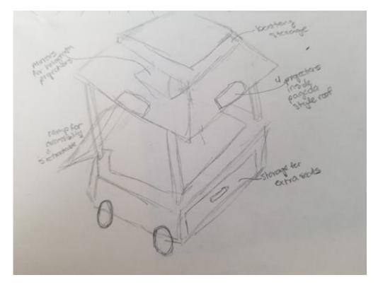
This design is a cart with a roof to protect from rain and block some sunlight. It includes some storage compartments for the seats, a ramp to allow wheelchair access, a battery storage compartment overhead to power all the electronics, and projectors pointing towards all four directions.
